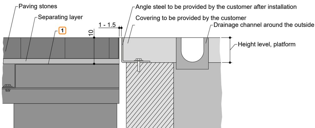
1 Sealing of the pit (see "Detail of building configuration - pit sealing", page 8)
